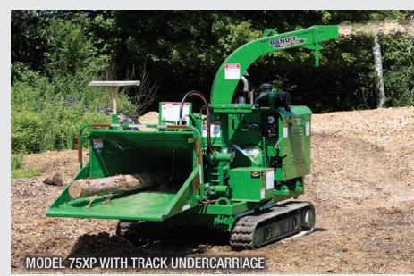
Track undercarriages are available for any Bandit hand-fed chipper! These units are extremely popular for land clearing, fire mitigation, and remote jobs where towable chippers can't reach.
